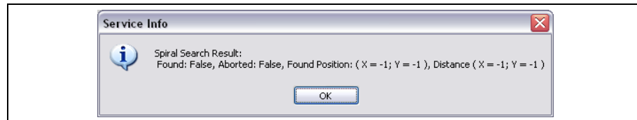
Fig. 426: Spiral Search Result - fiducial not found
